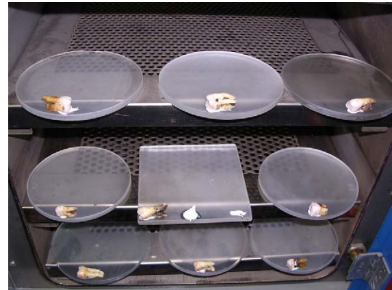
Fig. 4. Test samples placed in Anglis dry heat oven. The position of each sample was tested with the Pet-Scan II interrogator, so that there was no read-out interference with the neighboring devices.
